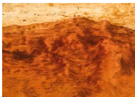
▲ The most widely used veneer is the rotary-cut form, more commonly known as kevasingo
